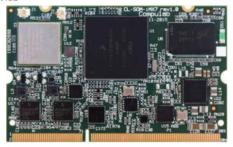
CL-SOM-iMX7 is a tiny Computer-on-Module (CoM) board built around Freescale i.MX7 and designed to serve as a building block in embedded applications.
