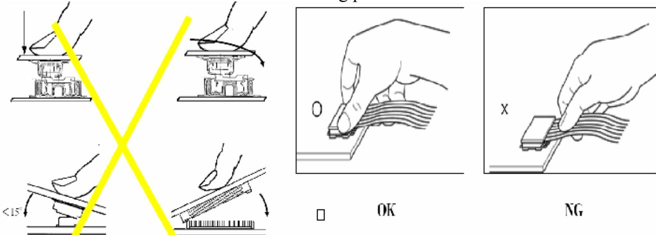
**Precaution for soldering to the LCM**
